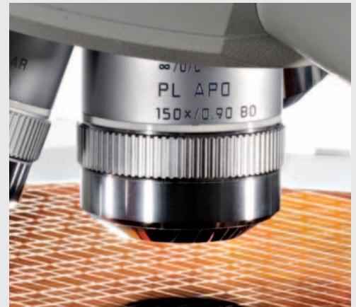
Multi-functional objective: HCX Plan APO 150x/0.90
