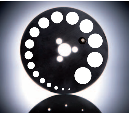
The 17-position aperture disk allows 100% reproducibility.
