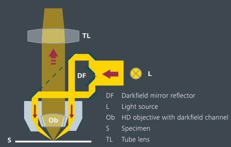
In Darkfield contrast, the sample is illuminated under an angle. As a result, only the diffracted light is detected and leaves the background dark. This method is particularly suitable for visualizing edges, scratches, and other surface topographies. In addition, semi-opaque phases are identified by its color. Compare the semi-opaque phase of copper oxide inclusions that appears in garnet red color in the image above.
