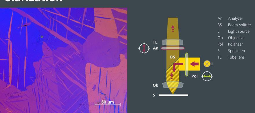
Polarized light is used in transmitted and reflected light to detect crystal-like (birefringent) structures within all types of samples. When polarized light interacts with a sample, the polarization direction of the light is influenced. This effect can be used to visualize domains of different crystalline orientation. The image above shows a zinc sample – a material used in corrosion protection. A polarizer and an analyzer are required to perform polarization microscopy.
