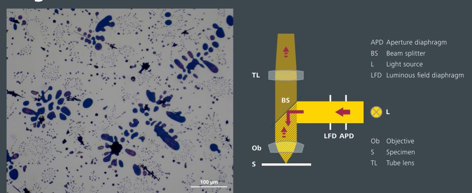
Brightfield contrast is the most common contrast method in light microscopy. Details of a sample are distinguished by the different reflectance of the materials in the specimen. This generates the typical image of a dark or colored sample on a bright background. Compare the above image of copper with oxide.
