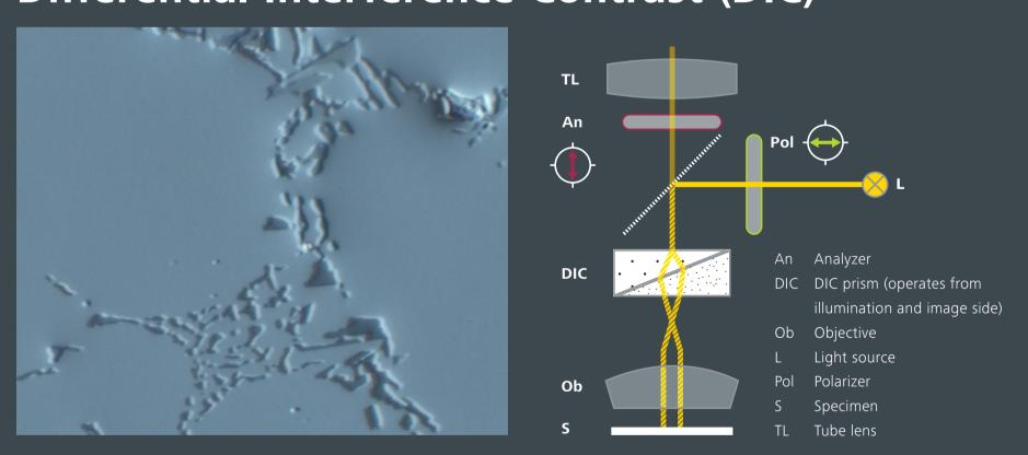
DIC is the most common method to visualize surface topography such as slopes, valleys, and other discontinuities or to check surfaces for defects, natural or preparation induced. It adds contrast to the image by evaluating the optical path length difference at surface structures using interferometry. DIC enables the visualization of even small surface structures due to the slightly dissimilar optical path length in the object. Compare the image of cast aluminum above.
