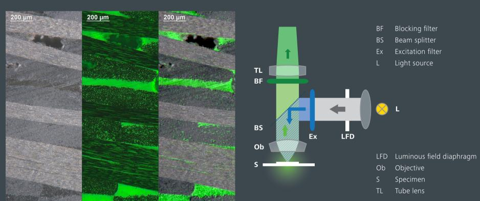
Fluorescence contrast is used in various applications like failure analysis, defect location or material analysis. Materials with fluorescence properties absorb light of a certain wavelength and emit it again at a different wavelength. The image above shows a carbon reinforced composite where specific areas, here the polymer matrix, are made visible with fluorescence. This technique requires a capable light source, filters to specify and separate your excitation and emission light, and a camera.
